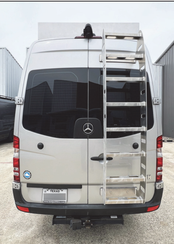
Ladder for Roof Access
