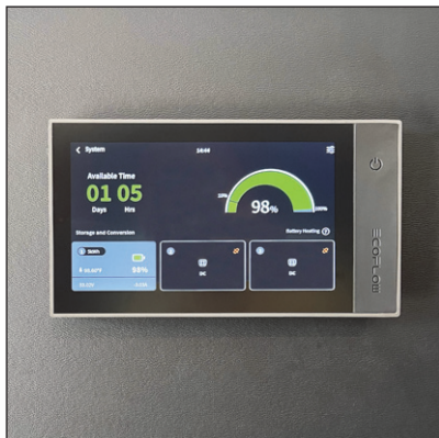
Power System Controller
