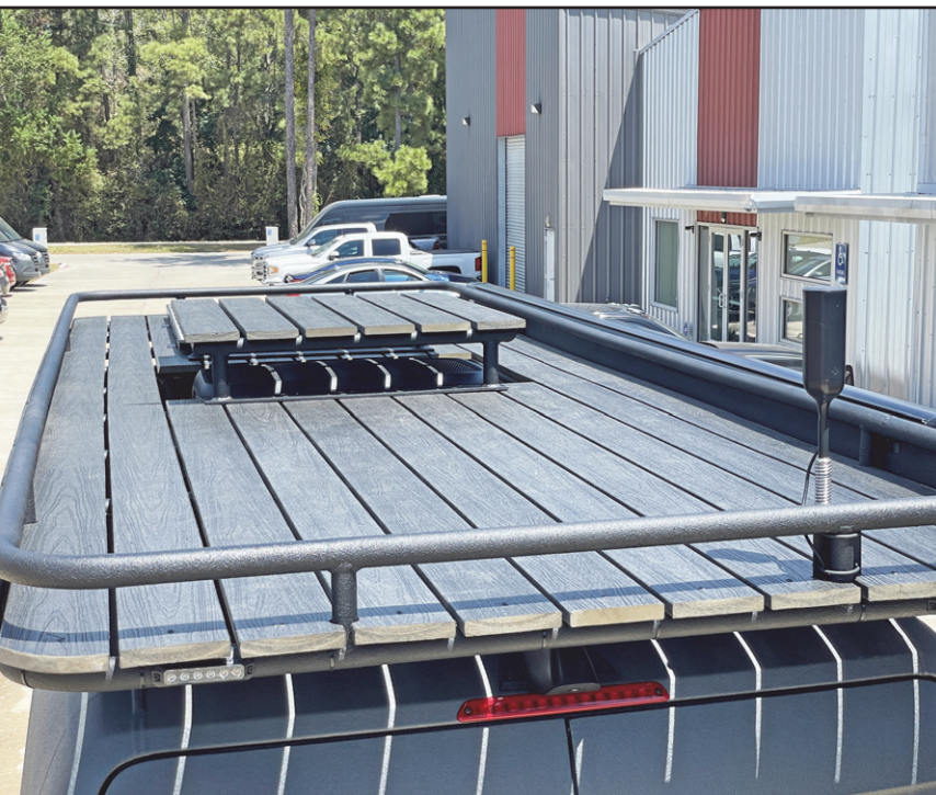
Roof Deck with Cell Phone Signal Booster
