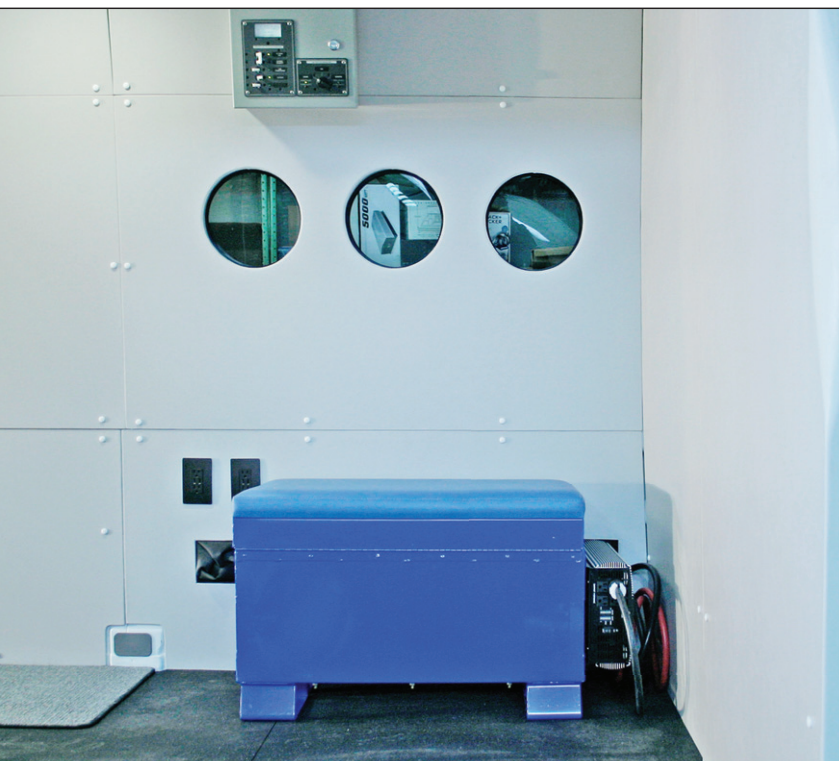
Porthole Windows and Battery Box
