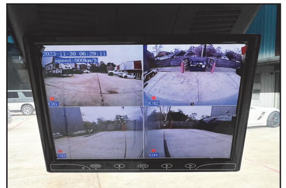
Four Camera Security System
